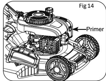
2. Stand behind the mower . Pull the engine Start/ stop lever toward upper handle With one hand . And Place the other hand On the starter handle.
